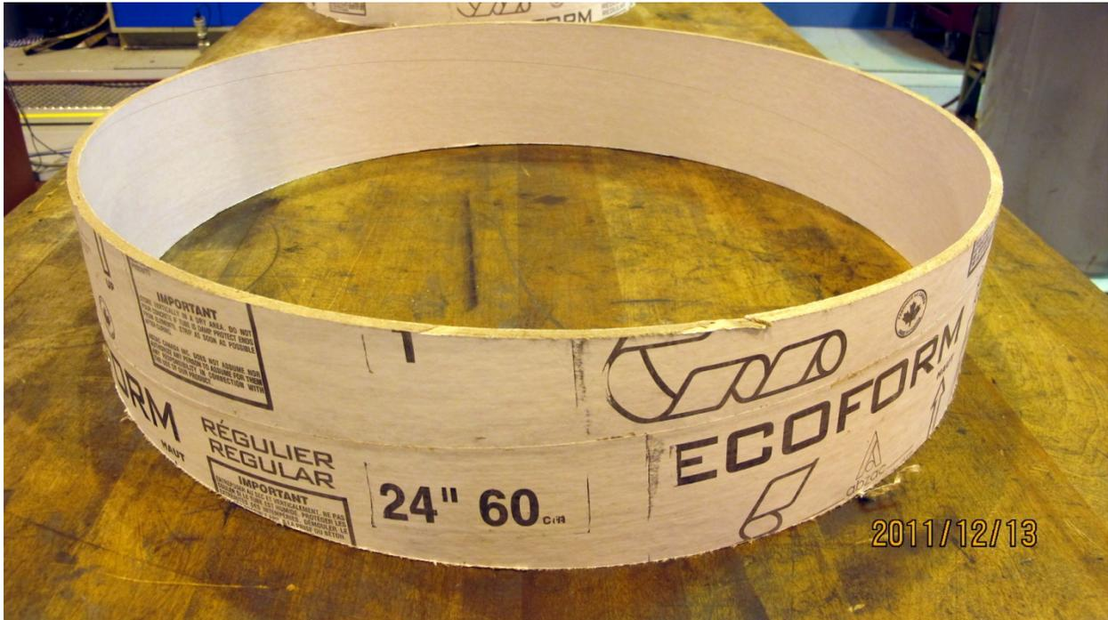
Picture A.3 – Typical 1/4 inch thick 5 inch wide sample
