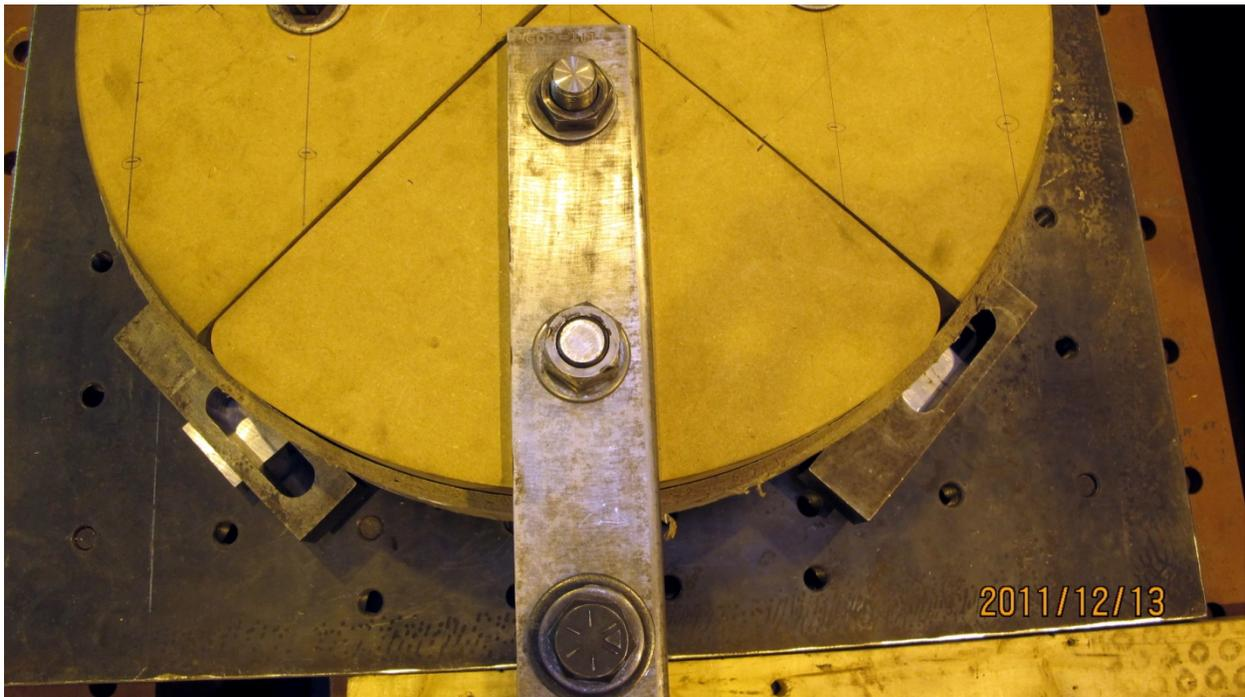
Picture A.10 – Sample installation prior to a test, typical, shown with a 1/2 inch thick sample
