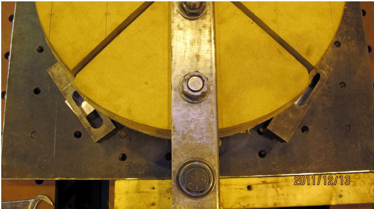
Picture A.12 – Typical sample deformation under loading, 1/2 inch thick sample shown
