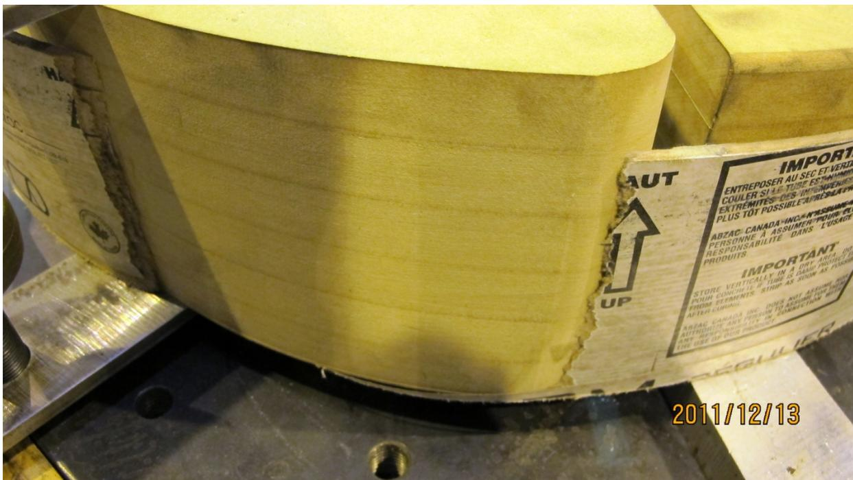
Picture A.14 – Typical breakage, 1/8 inch thick sample shown
