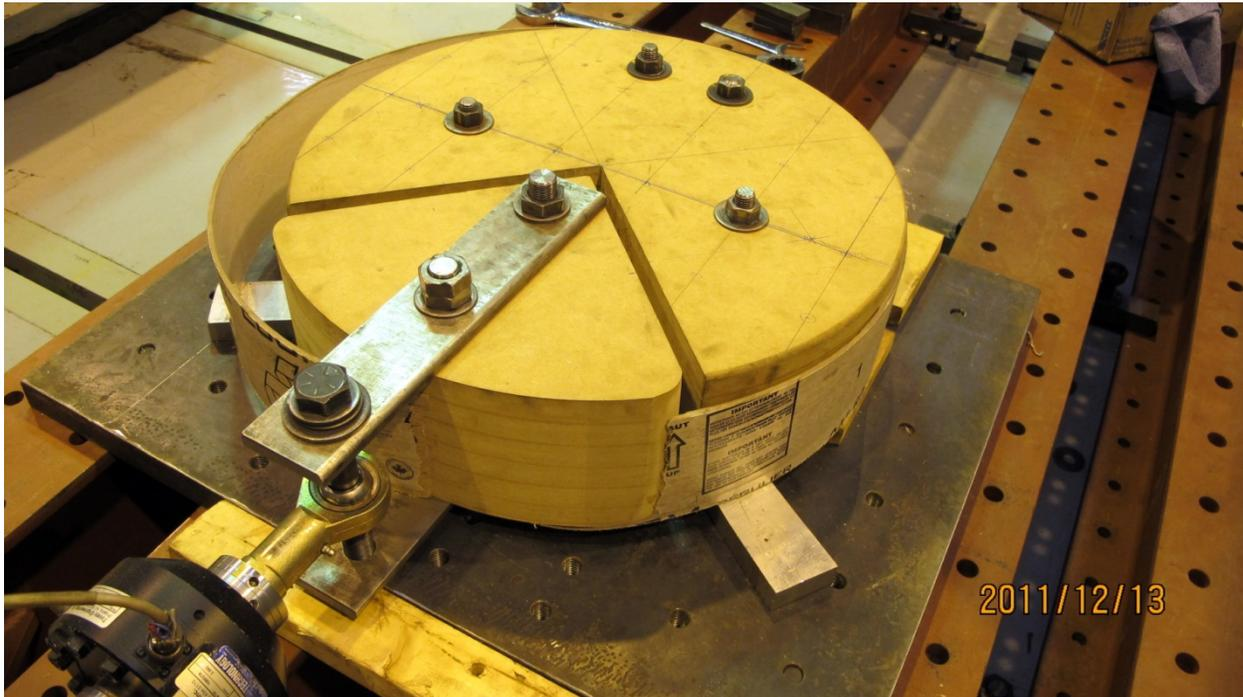
Picture A.13 – Typical breakage, 1/8 inch thick sample shown
