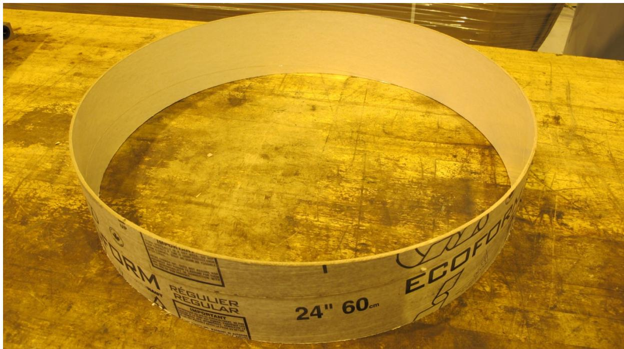
Picture A.2 – Typical 1/8 inch thick 5 inch wide sample
