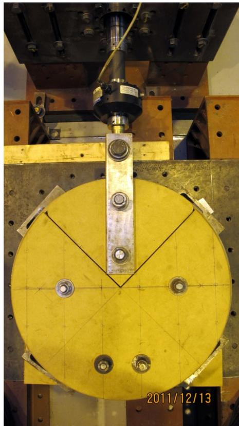
Picture A.9 – Sample installation prior to a test, typical, shown with a 1/2 inch thick sample
